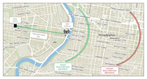
The recommended method for plotting TA arcs associated with urban outdoor DAS deployments – at least, as far as T-Mobile outdoor DAS sites are concerned – is to estimate or determine the length of the fibre connection between the central base station and the DAS antenna, to subtract this distance from the inferred TA distance and to plot the remainder from the antenna as a TA arc.
