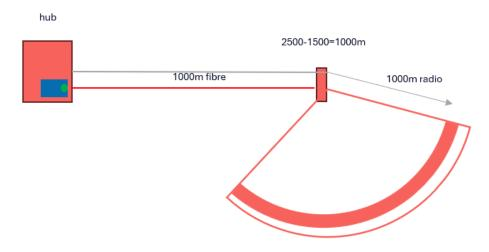
If the exact length of each fibre connection was known, it would be possible to compensate for the additional delay – by multiplying the exact fibre length by 1.5 before subtracting that value from the inferred TA distance.
