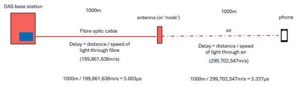
An example of the effect of the slower transit of light through fibre is shown in the diagram. The symbol  $\mu s$  represents microseconds.
