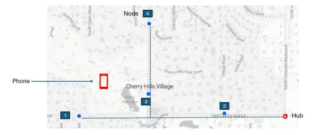
Let's imagine that a phone (in red) is situated in an area where it could connect to any of three nearby nodes (1, 3 or 4). It will be receiving copies of the same signal from all three nodes on the downlink, and those nodes will be receiving copies of the same uplink signal and passing it back to the base station (which is presumably in the hub).
