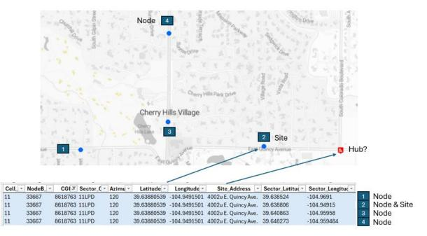
LTE Cell ID 310-260-8618763 is listed four times in the tower list, with the same site address, the same site lat/long but different sector lat/long details. The obvious assumption to make is that the site address and site lat/long relate to the hub and the various sector locations are the nodes.
