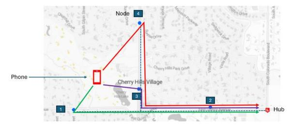
The base station will calculate TA from whichever is the dominant version of the signal from moment to moment. If the signal routed via node 1 is used to calculate TA, there will be a lower amount of delay than if the signal routed via node 4 was used.
