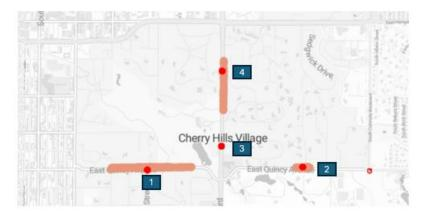
The orange areas on the map above show where that cell ID was detected as providing serving coverage during the RF survey.
