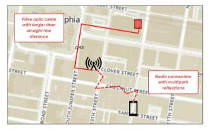
Firstly, if the fibre cable between a specific DAS antenna and the base station follows a direct path, then the delay suffered by cellular signals will be roughly comparable to the straight-line distance between those elements (albeit with slightly more delay as light travels more slowly through glass than through air).
