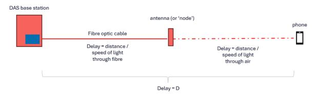
Light moves through fibre at a different speed than it moves through a vacuum or through air.
