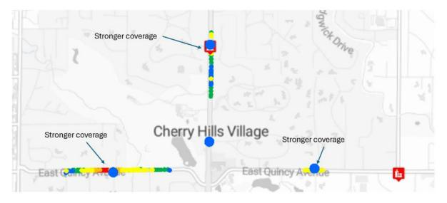
The localised nature of the RF coverage in the immediate vicinity of each node indicates that this isn't one coverage area from one antenna that covers the whole area, it is three separate coverage areas for the same cell ID.
