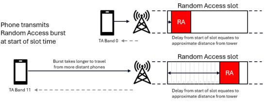
Initial TA band calculated from Random Access burst delay and sent to phone in Random Access Response
