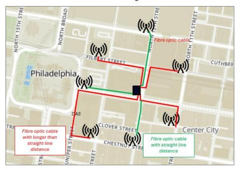
The base station is deployed at a central location. Antennas are deployed in neighbouring blocks, all served by radios installed at the central base station. Fibre optic cables link the base station to each antenna.
